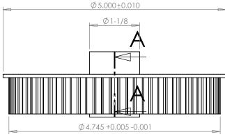
**NOTE: CORED PULLEYS** HAVE 1/16" THICK RIBS, REINFORCEMENT
